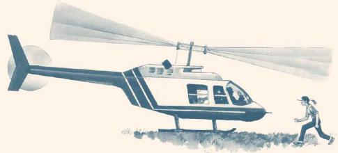
Before approaching the helicopter, communicate with the safety personnel on the ground and come into visual contact with the pilot. Approach and leave the helicopter in a bent position, always going towards the front with your head and eyes facing forward.
