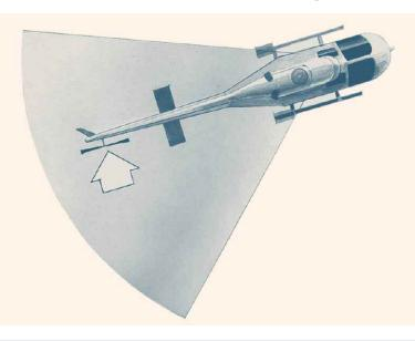
Never go around the rear of a helicopter or under its tail due to the risk of being caught by the rotor.
